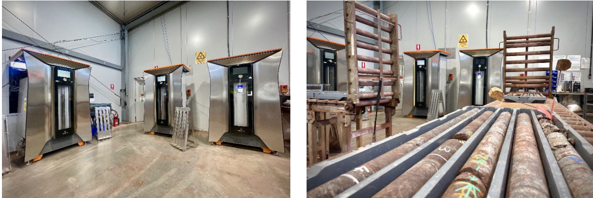
Figure 1 - Orexplore GeoCore X10® units at Carrapateena site
