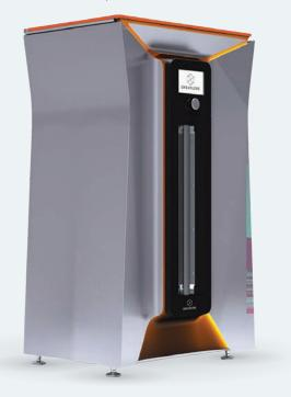
can generate core information, including structure, lithology, density, rock quality, and elements, which can be collected, interpreted and analysed. Each GeoCore X10<sup>®</sup>, scanning at less than 15 minutes per metre, can be combined in a configuration to keep up with your drill rigs, meaning that valuable results can be presented through the Orexplore Insight<sup>®</sup> software only hours after the core is drilled.
