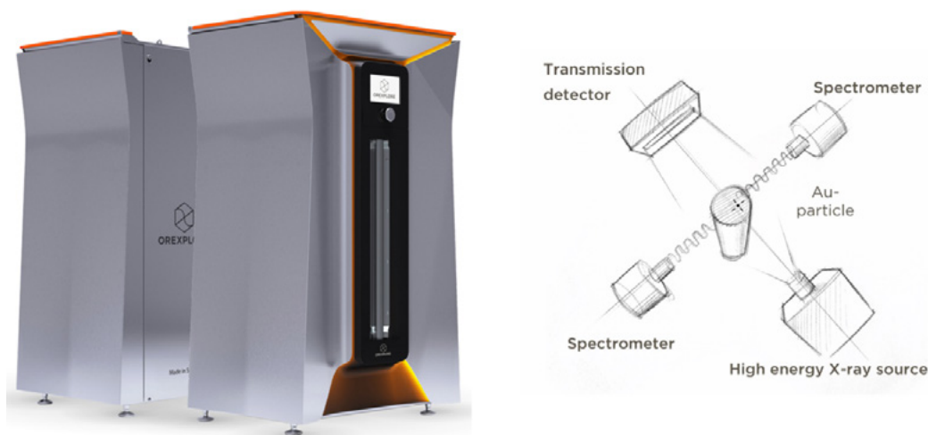
Figure 6 - GeoCore X10® and key internal instrumentation
